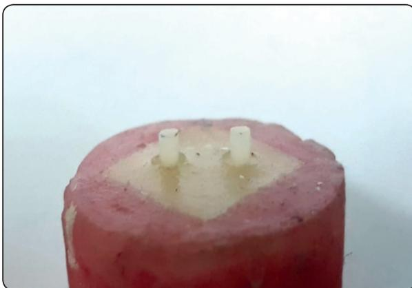
Fig. (1) Microcylinders prepared on each specimen for microshear bond strength testing.
