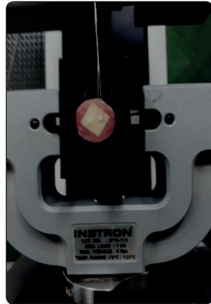
Fig. (2) Specimen mounted on Universal Testing Machine for microshear bond strength testing.
