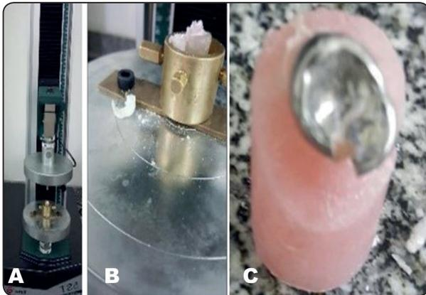
Fig. (8): a. Universal testing machine, b. fractured Figaro crown, c. fractured SSC.
