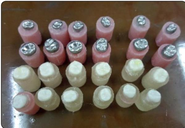
Fig. (1): Showing the 24 specimens crowns cemented on their acrylic die.
