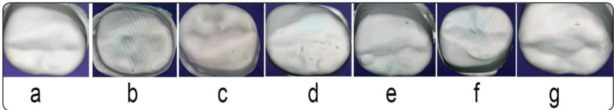
Fig. (2): images showing the deformity and wear in Figaro crown “D Mrduim”: a. before cyclic loading, b-g. after the cyclic loading
