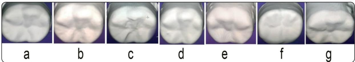
Fig. (3): Images showing the deformity and wear in Figaro crown “E Mrduim”: a. before cyclic loading, b-g. after the cyclic loading.
