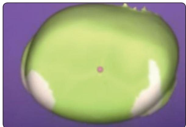
Fig. (7): Superimposed image of stainless steel crown showing areas of 3-D wear in white color compared to original dimensions in green.
