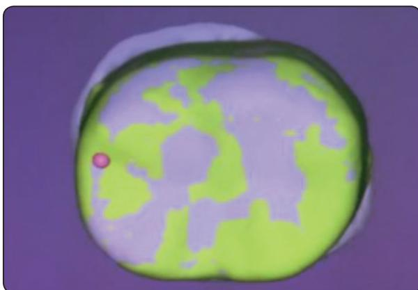
Fig. (6): Superimposed image of Figaro crown showing areas of 3-D wear in white color compared to original dimensions in green.
