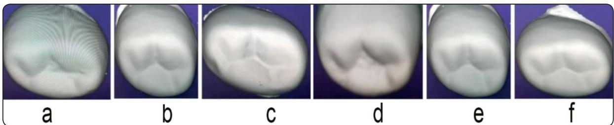
Fig. (4): Images showing SSC crown “D 4”: a. before cyclic loading, b-f. after the cyclic loading
