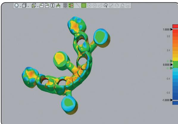
Fig. (4) 3d comparison between 3D printed and designed prosthesis
