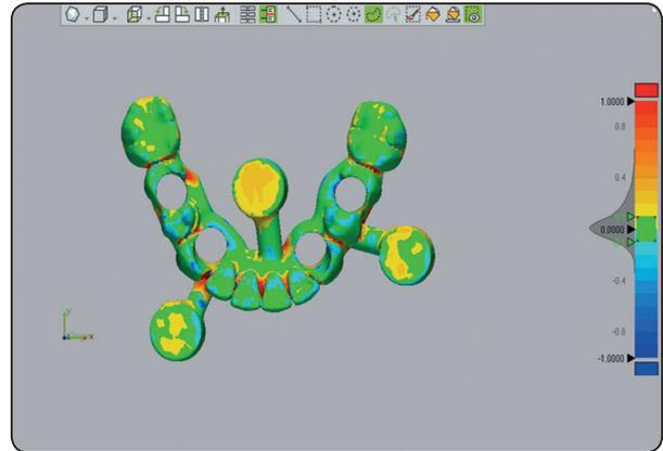
Fig. (5) 3d comparison between milled and designed prosthesis
