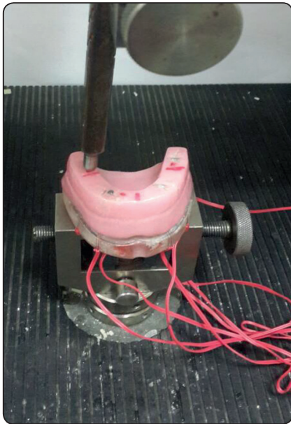
Fig (4). Unilateral loading using the loading pin of the universal testing machine
