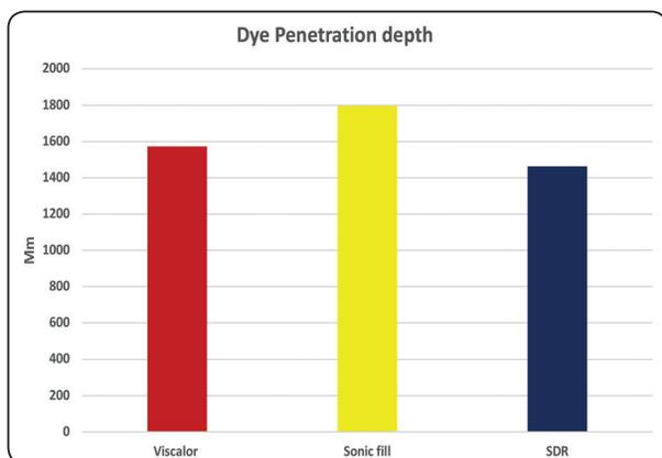
Fig. (7): Bar chart representing the dye penetration depth in Mm for the three tested composites.
