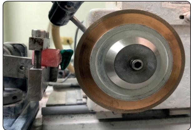
Fig. (5): Tooth sectioning into two halves using a micro slicing machine.
