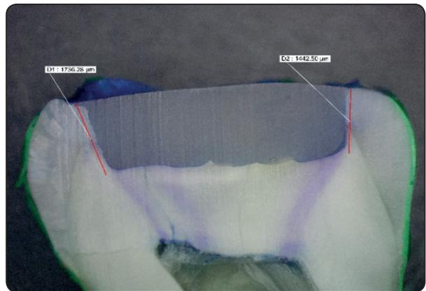
Fig. (6): Determining the depth of dye penetration using the image analysis software.
