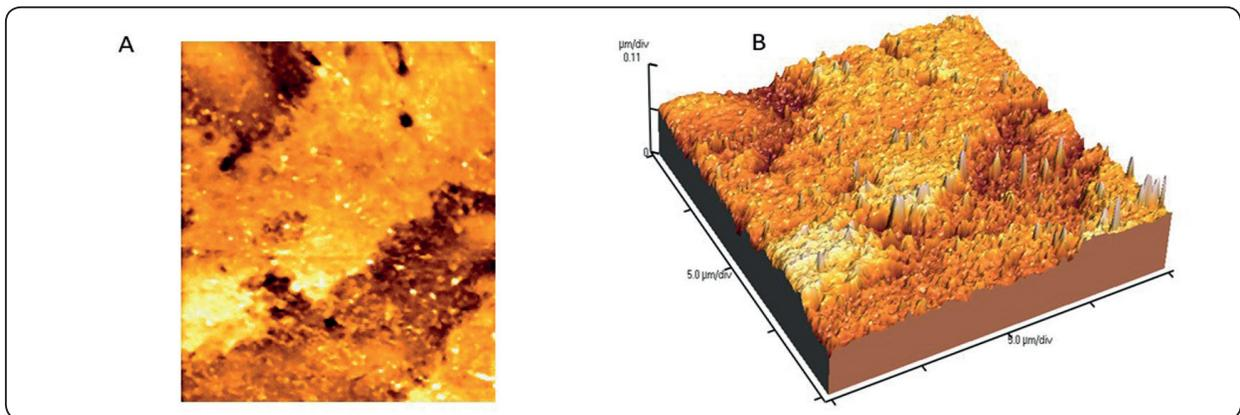
Fig. (2) AFM image of preheated Ceram X Duo resin composite (A) 2D image; (B) 3D image
