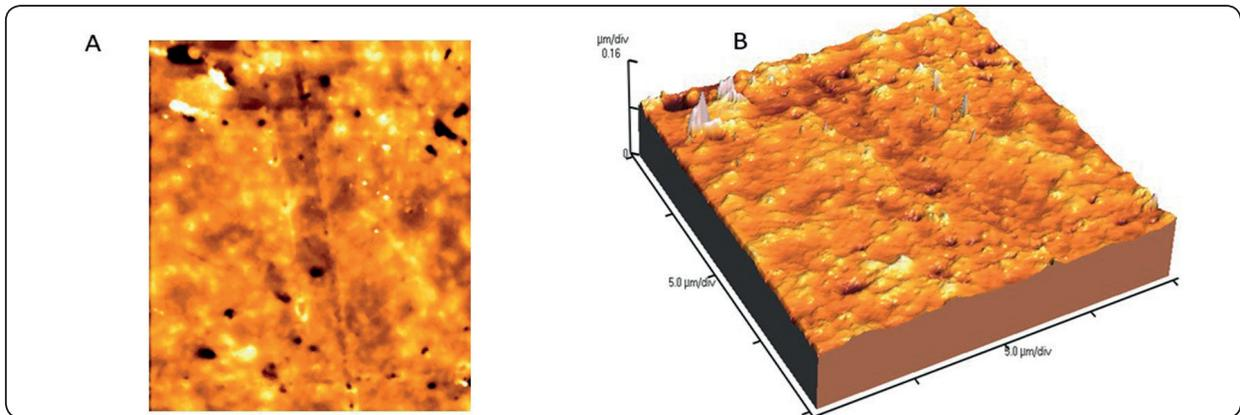
Fig. (1) AFM image of non-heated Ceram X Duo resin composite (A) 2D image; (B) 3D image
