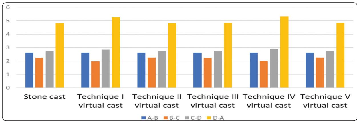
Fig. (9): comparison between the linear measurements made from one implant site to its successive on the stone cast and on the virtual models generated from the digital impressions.
