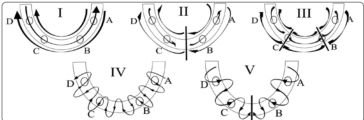
Fig. (3): Different scanning techniques used around implants positions A, B, C, and D. (I) full arch straight motion, (II) half arch straight motion, (III) sextant straight motion, (IV) full arch zigzag motion, (V) half arch zigzag motion.
