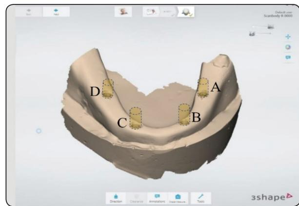
Fig. (7): A scan of the stone cast and its embedded implant analogues with sites of the cylindrical projections over each implant site.
