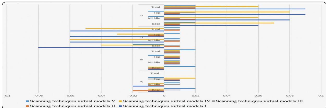
Fig. (10): Average horizontal deviations of the base, middle, top and whole of the cylinders superimposed on each implant sites A, B, C, and D as detected from the superimposition of the stone cast scan and the virtual models.
