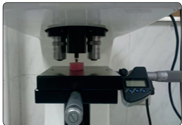
Fig. (1) Specimen placed in microhardness testing machine
