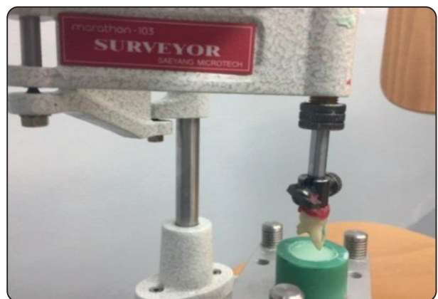
Fig. (1): Specimen fixed by sticky wax to the moving rod of the Mounting Surveyor
