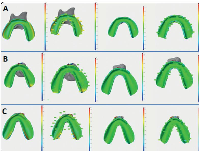
Fig. 5 (A,B,C): Assessment of denture base deformation for square, ovoid and tapered arch form respectively
