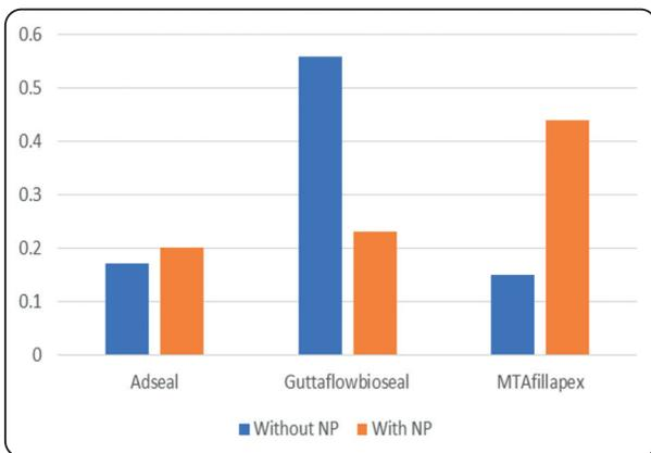
Fig. (1) Bar chart showing values for film thickness (mm) with and without NP addition.
