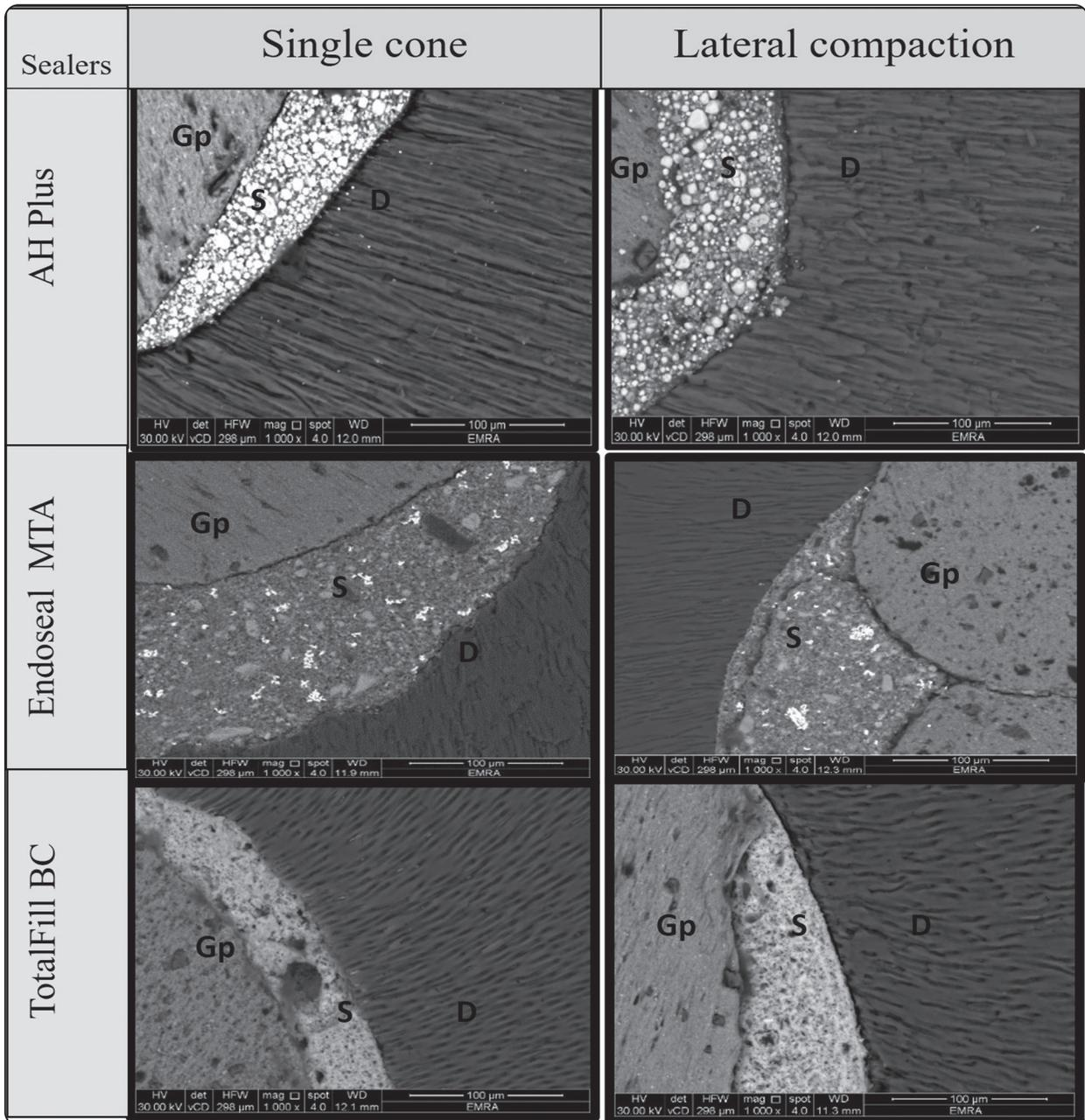
Fig. (5): Representative SEM photomicrographs showing interfacial adaptation of three tested sealers (S) with dentin (D) and gutta percha (GP) using the single cone (SC) and lateral compaction (LC) obturation techniques.
