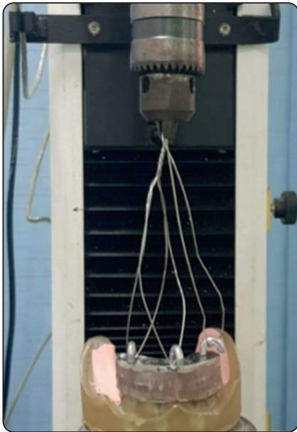
Fig. (4): Recording of retention using the universal testing machine
