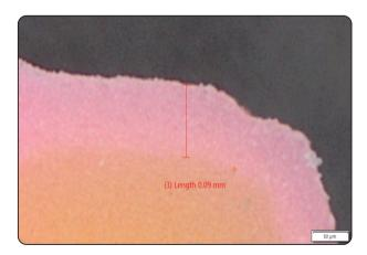
Fig. (4): Measurement of the gap distance (Pink silicone) thickness by Stereo Microscope
