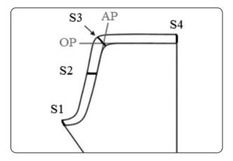
Fig. (3): Areas of measurements S1. Marginal gap, S2. Middle of Axial wall, S3. Axio-occlusal angle, and S4. Occlusal area, OP. Occlusal plane, AP. Axial plane.
