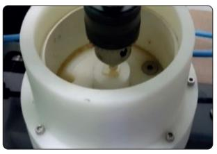
Fig. (2): Ceramic sample embedded in Teflon housing
