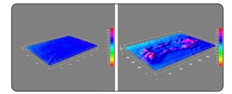
Fig. (5): Three-dimensional surface topography of VITA Enamic sample before and after chewing simulation
