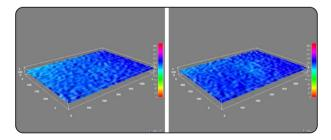
Fig. (7): Three-dimensional surface topography of VITA Suprinity sample before and after chewing simulation
