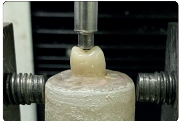
Fig. (3) Restored tooth fixed to the mount ready for fracture testing
