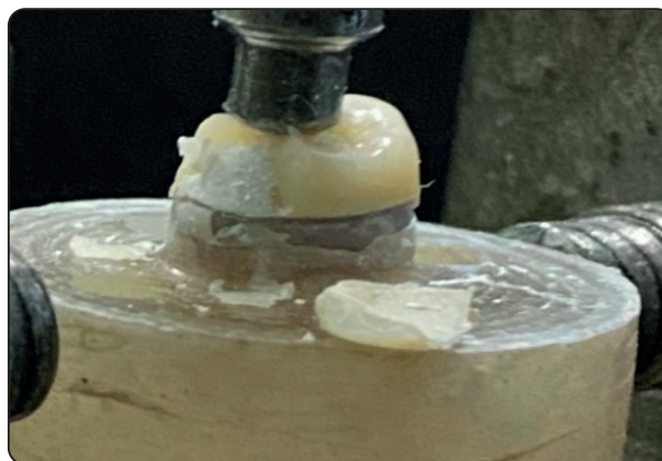
Fig. (5) PEEK endocrown restored sample after fracture resistance test with veneering composite debonding from core
