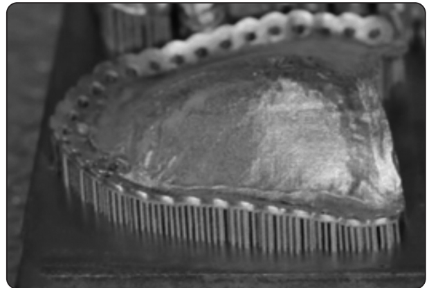
Fig. (4). The 3D printing of the metal palatal plate
