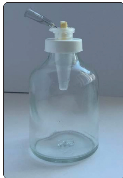
Fig. (1): Assembly for apical extrusion of debris
