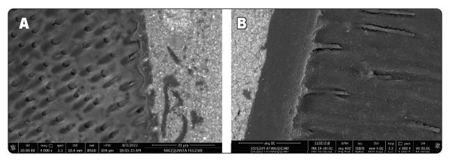
Fig. (8) and b; tooth restoration interface for non treated dentin at x 1500 magnification
