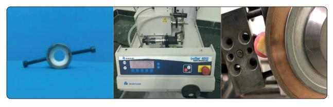
Fig. (1): Teflon mold with corresponding metal ring and paralleling screws (Top view)
