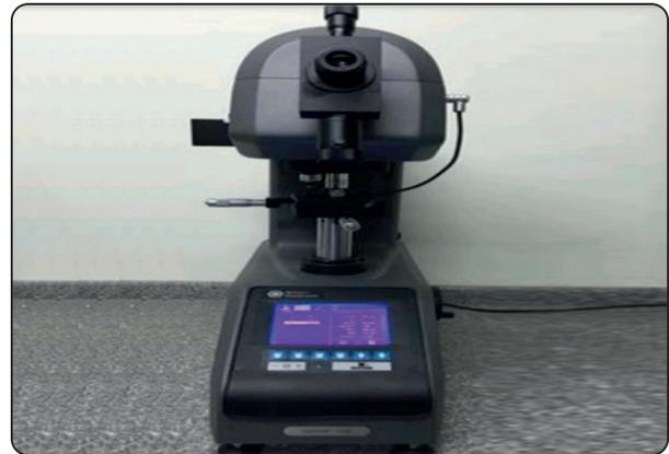
Fig. (2): Vickers Microhardness tester with diamond indenter.
