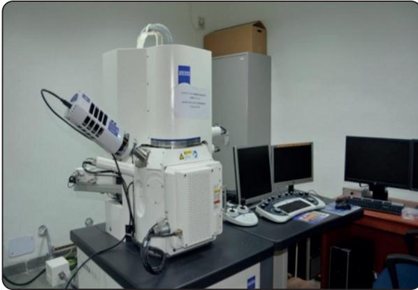
Fig. (3) Scanning electron microscope, surface topography
