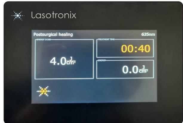
Fig. (1) 635 nm diode laser used in the study (Smart M, Lasotronix, poland)
