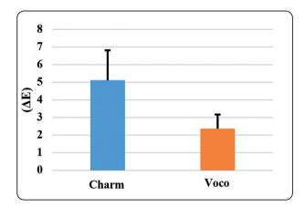
Figure 4: Histogram compared the mean colour change ( $\Delta E$ ) of two provisional materials.
