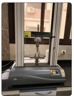
Fig. (2) Specimen in Universal testing machine for measuring flexural strength
