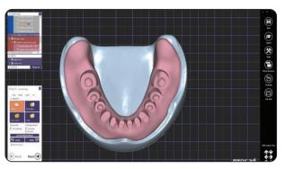
Fig. (2) Designing of lower complete denture base on Exocad software
