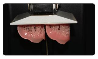
Fig. (3) Printing of two dentures bases at same cycle
