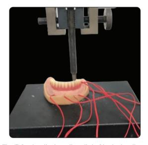
Fig. (7) Load application unilaterally by I bar load applicator
