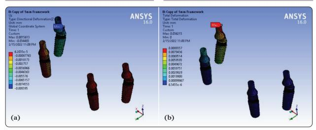
Fig. (3) Implant system results; (a) vertical deformation, (b) total deformation,
