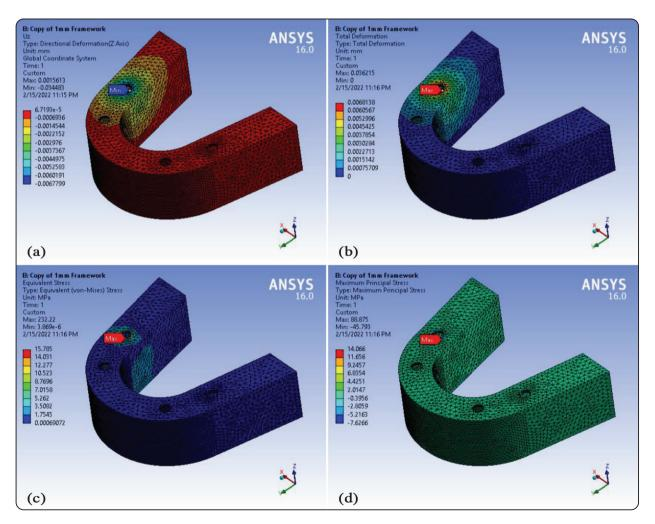
Fig. (2) Cortical bone results; (a) vertical deformation, (b) total deformation, (c) Von Mises stress,
