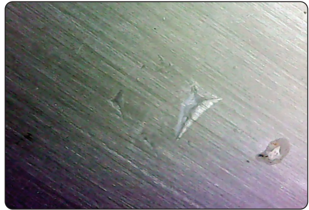
Fig. (1) Indentation mark left by the Vickers diamond indenter.
