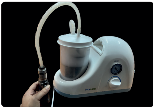
Fig. (3) A single EC device omitting aerosol to expose the specimens to the fumes for 20 cycles
