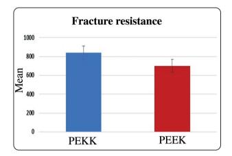
Fig (7): Boxplot representing maximum load of fracture resistance in both groups.
