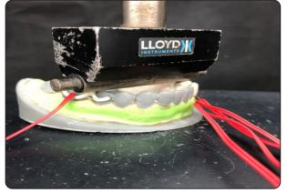
Fig (6): T-shaped load applicator was used to apply load bilaterally
