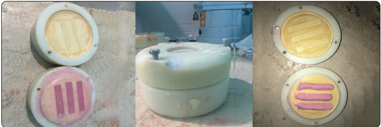
Fig. (4) a: Processed rectangle samples, b: Preparing closed flask for processing, c: Packing of acrylic mix in the flask
