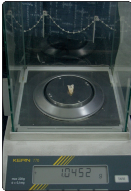
Fig. (1) A photograph showing: Sensitive digital scale were used to scale the samples (Kern 770, max= 220kg, KERN, Germany).
