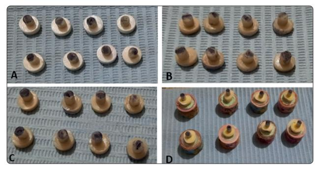
Fig. (1) The bonded ceramics to different core materials. A) Bonded ceramic to Zirconia. B) Bonded ceramic to RMGI. C)Bonded ceramic to composite resin. D) Bonded ceramic to flat dentin
