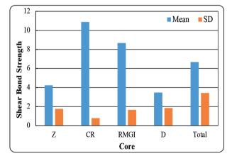
Fig. (2) Mean and standard deviation of shear bond strength of core materials. Z: Zirconia, CR: Composite Resin, RMGI: Resin-Modified Glass Ionomer, D: Dentin.
