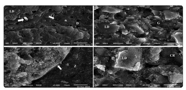
Fig. (4) SEM micrographs at x2000 showing the core/ceramic/resin interface characterization. (LD = Lithium disilicate glassceramic, CR = composite resin, D = Dentin, Z = zirconia, G = RMGI, 1 = odontoblastic process, 2 = opened dentinal tubules, 3 = resin cement).
