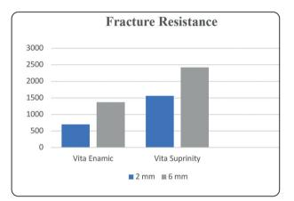
Fig. (1): Bar chart showing average fracture resistance (N) for different materials and preparation extensions (A)
