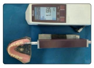
Fig. (8) Measuring the surface roughness for the acrylic dentures modified by Salinized Tio2 Nps)
