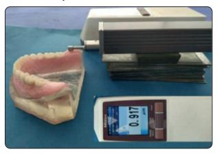
Fig. (7) Measuring the surface roughness for the acrylic dentures
