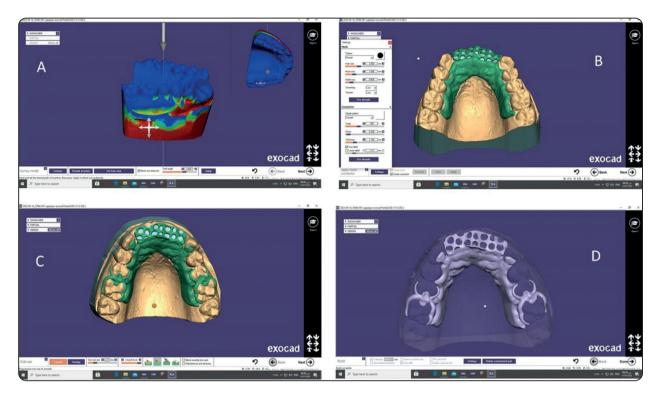
Fig. (1) A: Adjust the anteroposterior tilt and block out the undesirable undercuts. B: The outline of the design is marked. C: Finished design with the finish line.D: final framework design ready for printing the resin.
