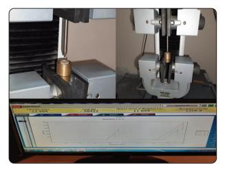
Fig. (3) Specimen placed centrally on three balls and loaded with piston till fracture.
