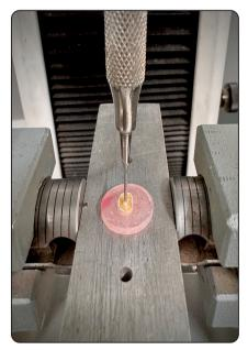
Fig. (1) Push out bond strength test
