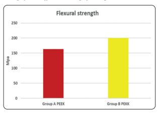
Fig. (4) Bar chart representing Flexural strength for different group.
