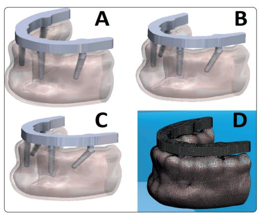
Fig. (1) a,b,c; models with the different angulations of posterior dental implant and d; meshing of the model
