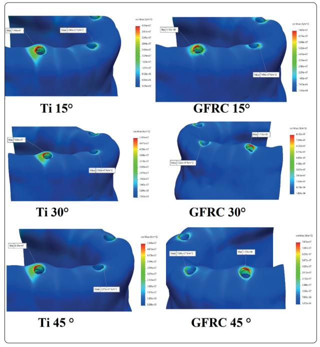
Fig. (2) Stress distribution patterns at the implant/crystal bone interface with six different models
