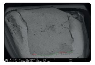
Fig. (1) SEM image (50×) and an example of the quantitative margin analysis. The green lines indicate continuous margin segments, and the red lines indicate noncontinuous margin segments
