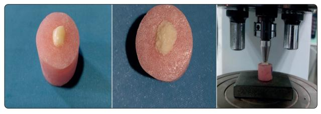
Fig. (1): Sample imbedded in acrylic
