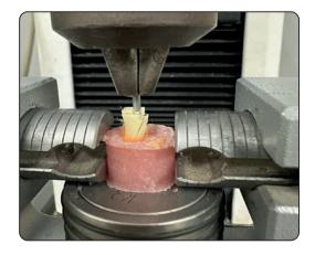
Fig. (1) Sample mounted on universal testing machine subjected to load until fracture.
