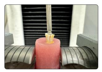
Fig. (1): Fracture resistance test setup.
