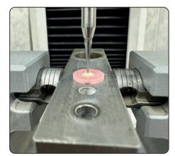
Fig. (4) A Slice Mounted in Universal Testing Machine.
