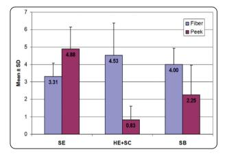
Fig. (6): Histogram presenting push-out bond strength of glass fiber and PEEK posts after different surface treatment methods.
