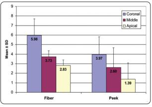
Fig. (8) Histogram showing push-out strength based on post type.
