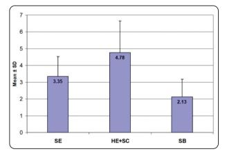
Fig. (9): Histogram presenting Push-out strength based on surface treatment method.
