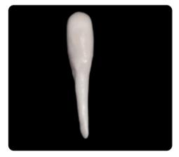
Fig. (2) Milled PEEK post with 10 mm in length.
