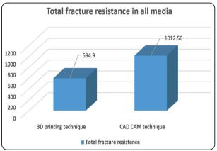
Figure (5) Total fracture resistance in all media
