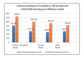
Fig. (4) Comparison of fracture resistance of samples in 3D printed technique and CAD/CAM techniques in different sub groups
