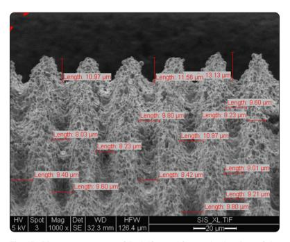
Fig. (4): Linear measurements of Rod #3, zone16, note that locations of the measurements were manually placed at almost the middle of each groove sloping wall.
