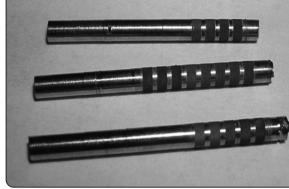
Fig. (1) Titanium rod laser micro-grooving set-up
