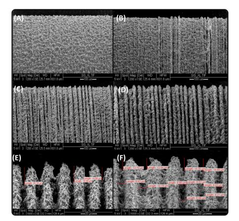
Fig. (3) SEM images with linear measurements recorded. A: Rod #1 zone 1. B: Rod #2, zone 5. C: Rod #2, zone 6. D: Rod #2, zone 11. E: Rod #2, zone 12. F: Rod #3, zone 14.
