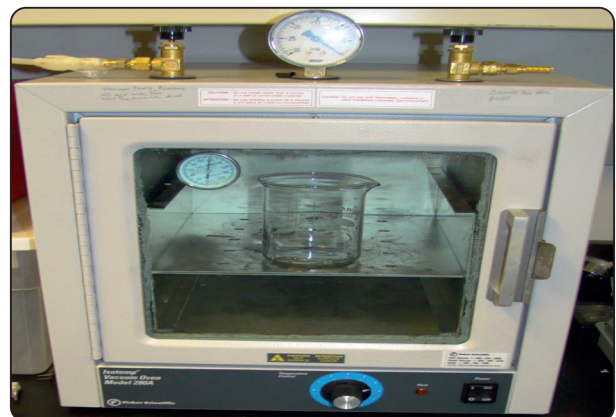
Fig. (2). Implants in the second method dried in dry heat oven for 5 hrs. at 30 °C.
