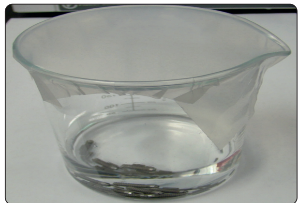
Fig. (3). The third method coated the implants by a layer of collagen, then immersion in RGD to solution.
