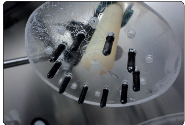
Fig. (1) The first coating method designed to suspend the implants in sequence of 3 solutions of alkane phosphonic acid, Maleimide, and finally Arg-Gly-Asp-Cys (RGDC).
