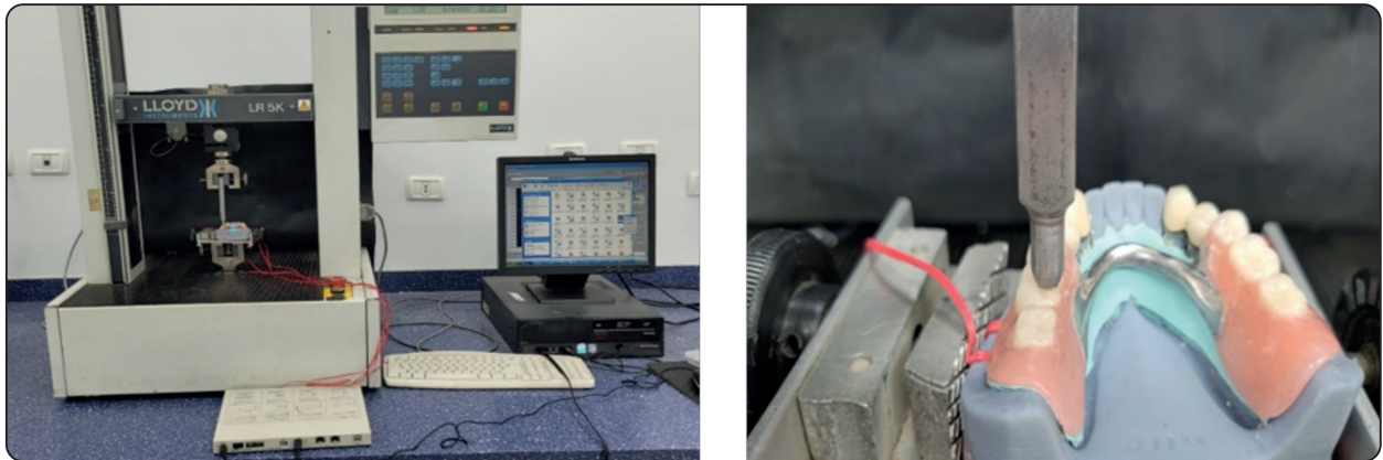
Fig. (10) Load application unilaterally on the RPD using the universal testing machine.
