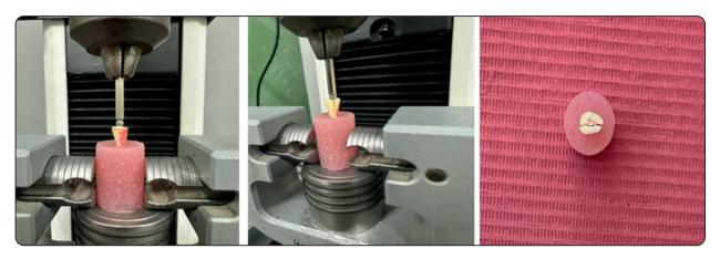
Fig. (1) Sample fracture after vertical loading with the Universal testing machine.
