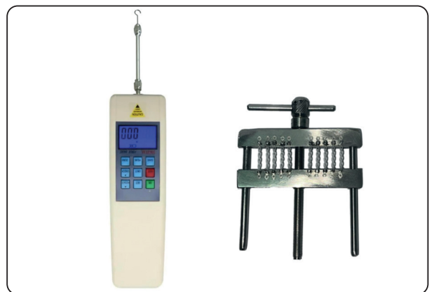
Fig. (2) Digital Force gauge and adjustable metal jig with stretched chains utilized in this study.
