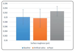
Fig. (2) Bar chart showing average surface roughness (µm) for baseline, artificial saliva and Pepsi
