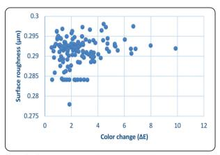
Fig. (3) Scatter plot showing the correlation between color change and surface roughness
